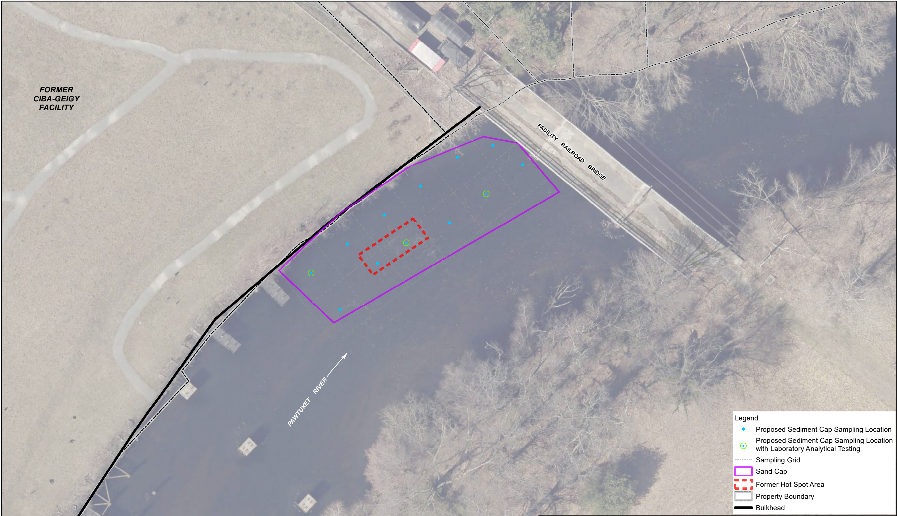
FIGURE 2 PROPOSED SEDIMENT CAP INSPECTION PLAN
